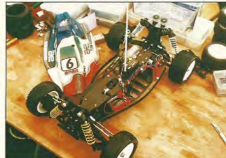
Craig Drescher's luck-less Cat 2000 was 'fully loaded' with carbon chassis parts, titanium everywhere and a chassis mounted Novak HPC.
